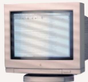
The effect of partially opened horizontal and vertical blinds on CRT screens
